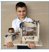
Rubber bands were used for their potential energy. When released, the rubber bands would cause magnets to spin, which would in turn cause electromagnetic induction. The process would create enough electricity to illuminate a string of holiday lights. It was a clean and simple way to create a small amount of electricity.
